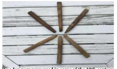
Wooden pegs were used in some of the 19th century covered bridges instead of nails. The bridge pegs were heavier than these, and were also used in older barns.
